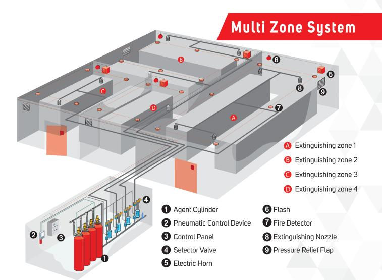
Multi zone system helps to save space & investment cost and it is easy extendable at any time. With 50 bar technology, it is possible to set up one multi-zone system instead of several single-zone systems. Multi-zone systems make use of a common, single stock of extinguishing agent for all rooms while, in the case of single-zone systems, a separate storage facility must be provided for each room. As such, multi-zone systems reduce costs and save space.
