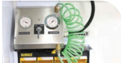
Extinguisher Pressurizing Unit
